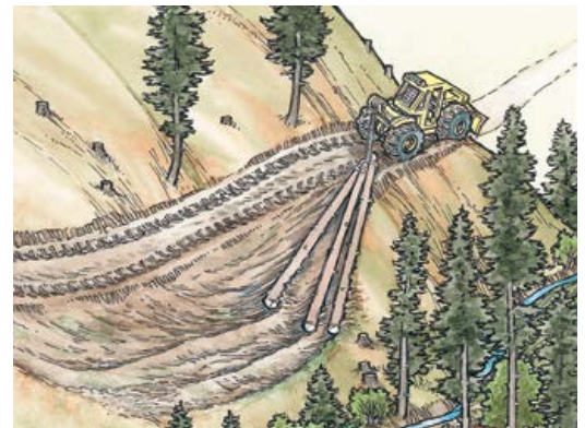
Both the logs and the yarding vehicle can cause excessive soil disturbance, especially on slopes.
