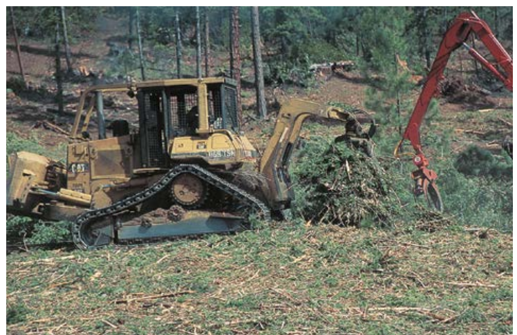
The same machine that brings whole trees to the landing may carry slash back and scatter it on the forest floor. This returns nutrients and organic matter to the soil for the next forest. It also protects soil from erosion, especially in skid trails. The fire hazard is minimal because the slash is crushed and close to the ground.
