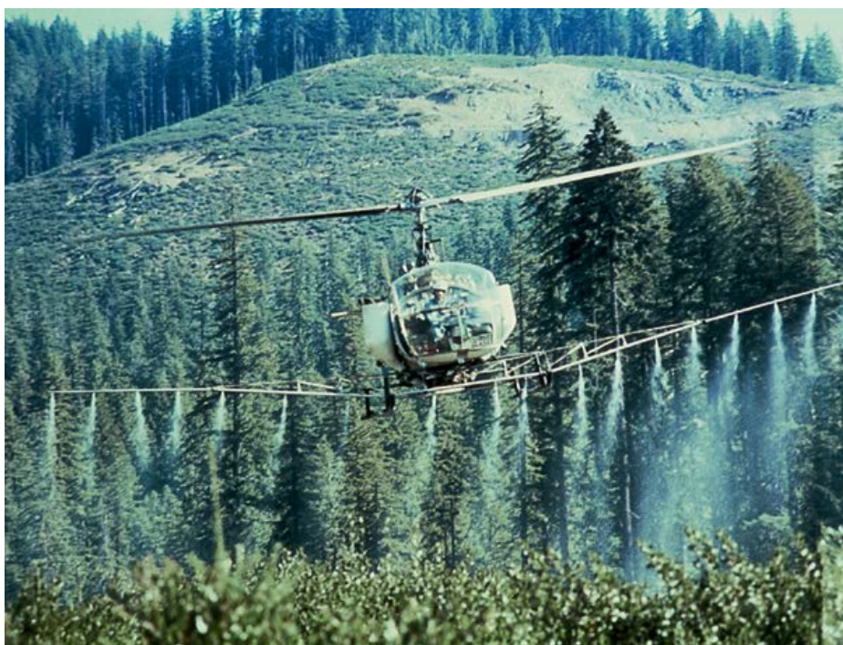
On larger forest ownerships, helicopters are a cost-effective method for applying herbicides.
