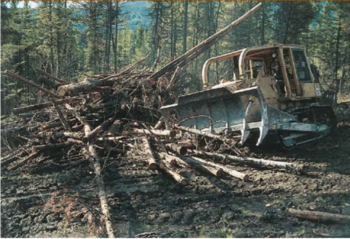
Crawler tractors with toothed brush blades are used to pile slash. Never use straight blades; they scrape the soil surface and carry soil into the slash pile. Piles free of soil burn cleaner, reduce soil erosion and protect productive topsoil.
