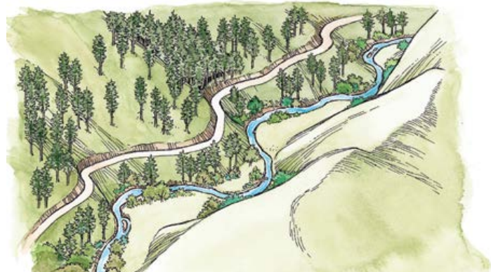
ACCEPTABLE OPTION, if no other alternative. Road built up on the 45 percent sideslopes. This option might be more difficult to build, but it is better.
