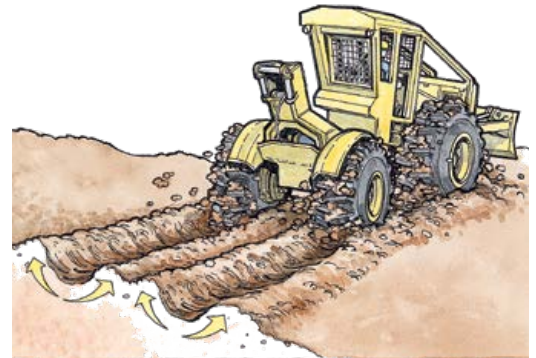
Major soil displacement is the lateral movement of soil, often producing ruts that can change natural drainage and increase erosion.
