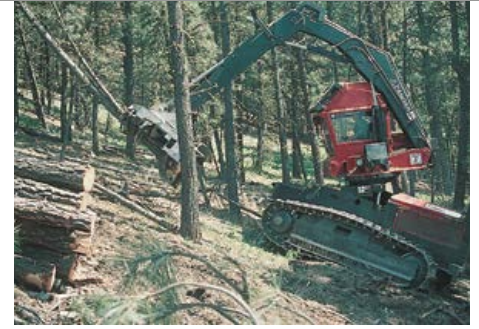
A feller-buncher severs trees and lays them in bunches with limbs and tops attached. Bunches are oriented with tree trunks facing downhill.
