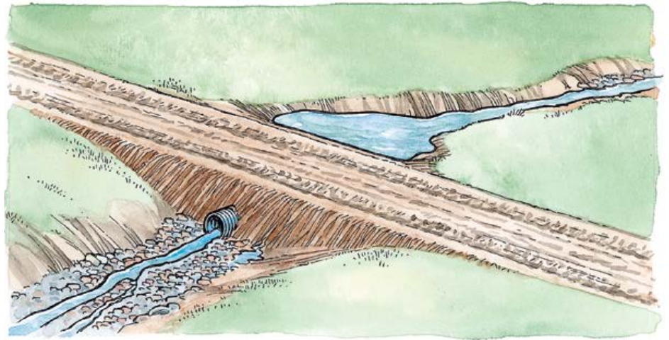
This temporary stream crossing culvert is too small. The stream is ponding behind the culvert and seeping through the fill. The culvert could fail, sending fill soil downstream.
