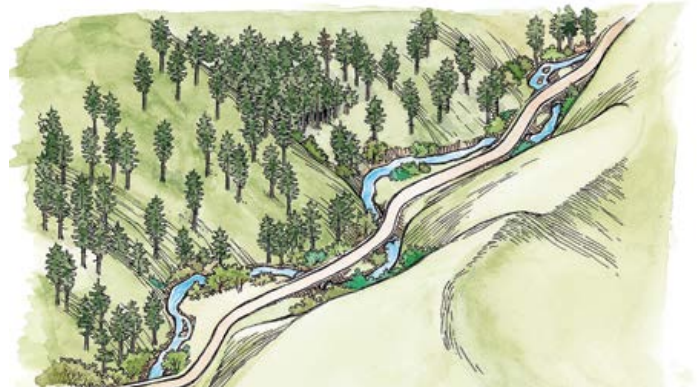
UNACCEPTABLE OPTION. Roads built or reconstructed next to a stream channel with multiple crossings are not allowed. Note: Many older roads and highways are in such locations.
