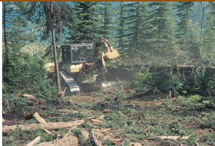
This crawler tractor, equipped with a grapple, picks up whole trees and moves them to a landing or roadside.
